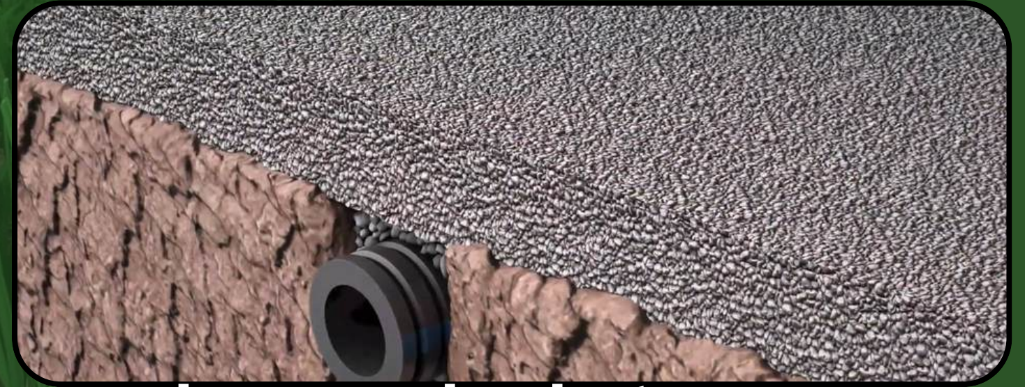
5– Fine Crushed Stone Layer
